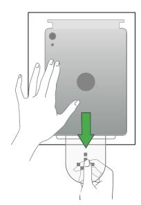
Hold the applicator firmly and pull out the tab marked "Pull Out".
